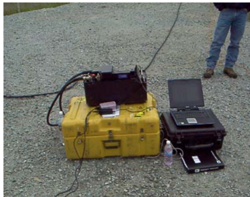
Figure 8: Laptop connected to 10-AU
