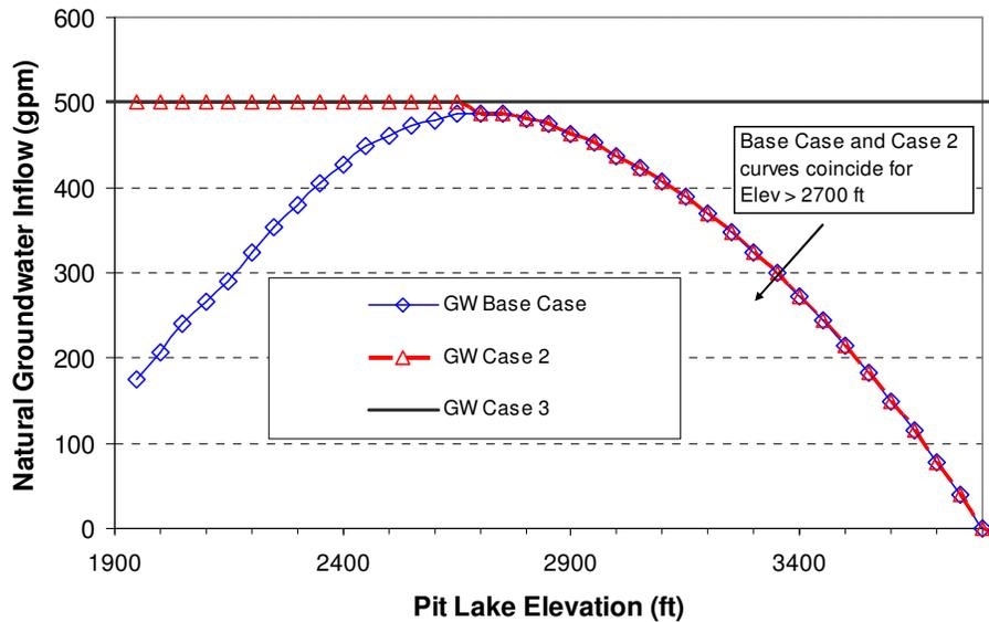
Figure 2. Rates of groundwater inflow used in model simulations.
