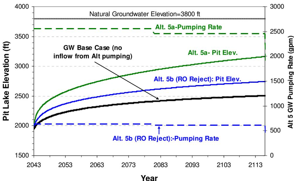
**Figure 5** Alternative 5 predicted rates of filling of the Sierrita pit lake. Dashed lines show the rate of groundwater pumping into the pit according to the schedules in Table 2 for Alternative 5a and Alternative 5b. The filling rate for the GW Base Case is shown for comparison.
