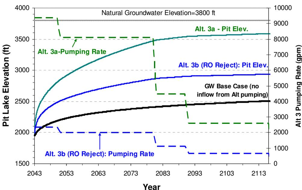
**Figure 4.** Alternative 3 predicted rates of filling of the Sierrita pit lake. Dashed lines show the rate of groundwater pumping into the pit according to the schedules in Table 2 for Alternative 3a and Alternative 3b. The filling rate for the GW Base Case is shown for comparison.
