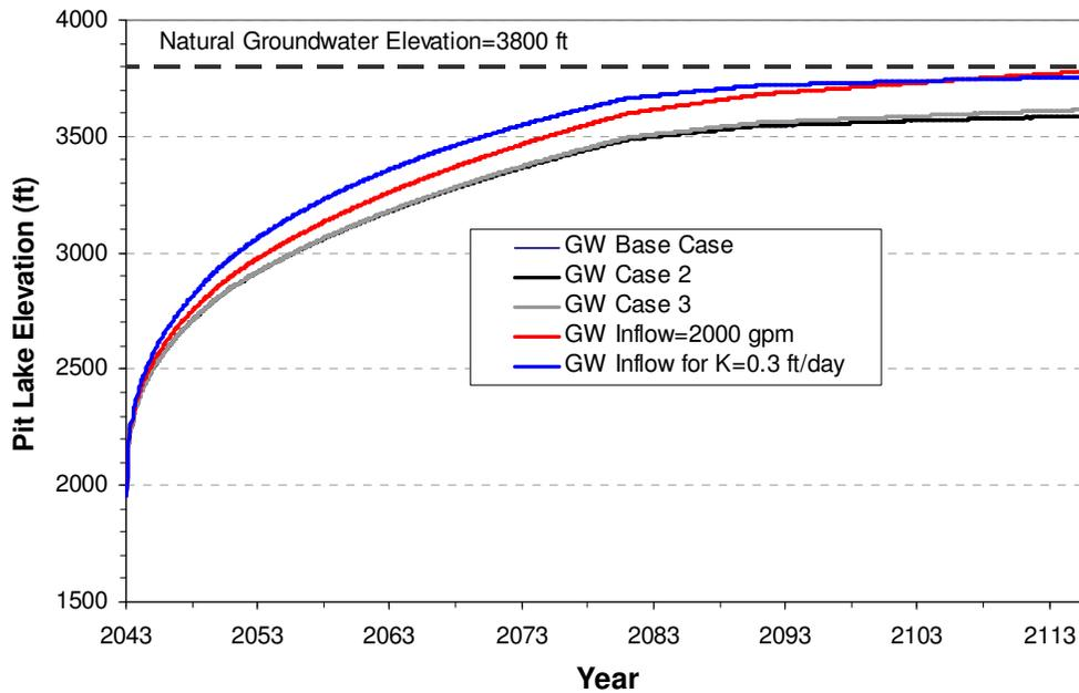
**Figure 6.** Sensitivity of the rate of pit lake filling to different methods of calculating natural groundwater inflow rates for the Alternative 3a mitigation pumping scenario. Data for GW Base Case and GW Case 2 overlap so only one line is shown.
