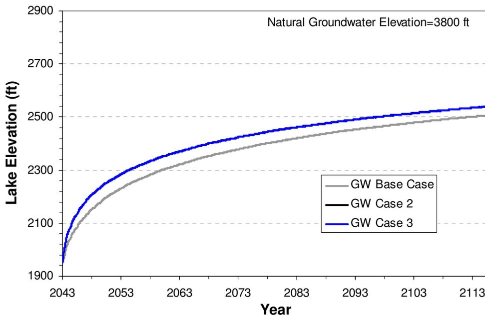
**Figure 3.** Based case predicted rates of filling of the Sierrita pit lake by natural inflows (no alternative pumping) for three representations of natural groundwater inflow. (Data for GW Case 2 and GW Case 3 are nearly equivalent so only one line is shown.)
