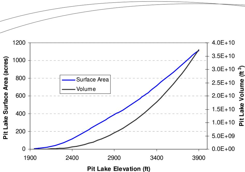
**Figure 1.** Surface area-elevation and volume-elevation curves for the Sierrita pit lake.
