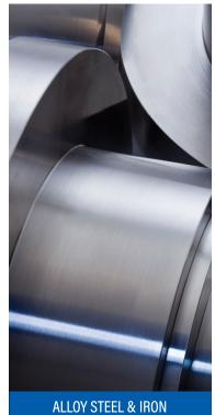
To increase hardness and wear resistance over a broad temperature, molybdenum is added to tool- and high-speed steel. It increases the strength and hardness of cast iron, as well as increases elevated temperature strength and creep resistance. In high-strength, low-alloy steels (HSLA) molybdenum improves strength and weldability.
