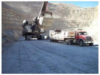
While moving a shovel with a motivator the motivator should be placed in a location uphill of the shovel in such a position that in the event of unintended shovel travel the motivator will not be in the potential path of travel.
