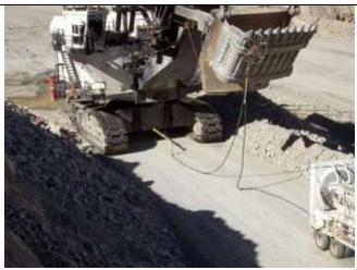
Proceed on grade with motivator safely positioned uphill of the shovel, regardless of the direction of travel. Spotters and other ground personnel shall be positioned 200 feet away to appropriately manage the move and avoid the potential hazard of fly metal generated by the shovel tracks. No one will be positioned to the sides or the downhill side of the shovel while in propel.
