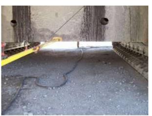
When positioning the motivator for a shovel move, ensure there is at least 50 feet between the shovel dipper's footprint and the tail of the motivator. While still connected to power and using the spotter, walk the shovel over the cable (which is connected to the motivator).
