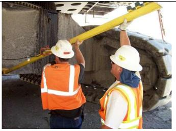
When needed for cable management, attach a temporary stinger to the front of shovel.
