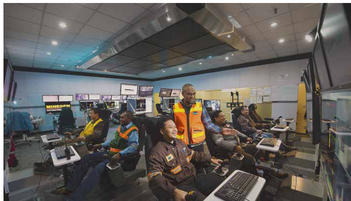
PTFI operators remotely pilot automated loaders from the underground mines control facility, maintaining worker safety and increased productivity.
