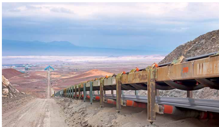
The gravitational potential energy associated with the 470-meter descent of El Abra's overland ore conveyor is greater than the power required to power the conveyor itself. As a result, during its braking, five megawatts of electricity is produced and used in operations.
