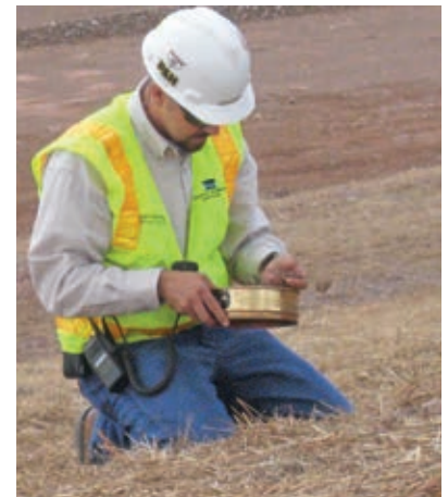
Quality assurance testing is performed to ensure seeding follows the prescribed application rate. During reclamation, once soil cover is down, mulch is placed on top, then seeded.
