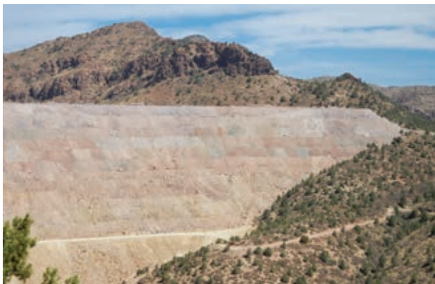
Before and after photos evaluating alternative cover material. Rock capping is tested for resistance to erosion, vegetation success and limiting water infiltration. In these 2012 photos, cover material was applied in February, seeded in June and vegetation growth reflected as of September.
