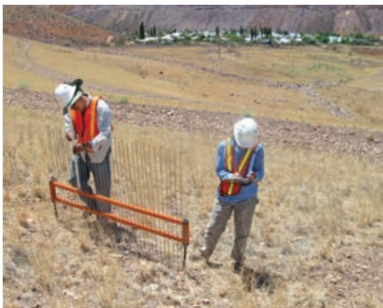
Workers analyze a mechanical erosionometer, which measures surface topography changes over time. This helps monitor success of existing cover material in mitigating erosion. Laser erosionimeters are also utilized.
