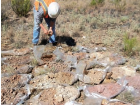
A worker analyzes a variety of cover material to determine which samples best aid with vegetation. Each bag represents 2 feet of material drilled from different locations. Certain plants have greater success with specific cover material.
