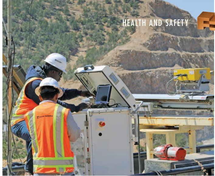
Geomechanical engineers use instruments such as radar and GPS to detect conditions that could lead to pit slope failure. Above, Engineers Caesar Oppong and Enrique Silva calibrate a radar unit that scans for slope movement at Tyrone operations.
