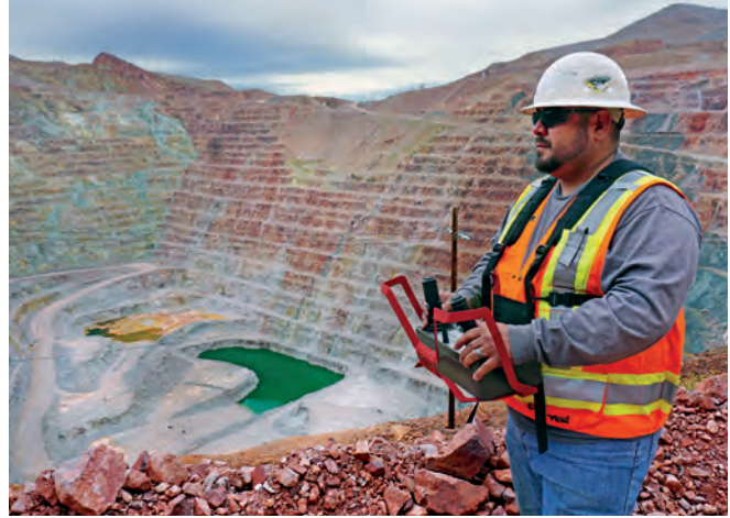
The application of remote-controlled equipment allows operators to remain at a safe distance. Operator Pete Rosales remotely controls a skid steer loader at the Garfield pit in Morenci, Arizona.
