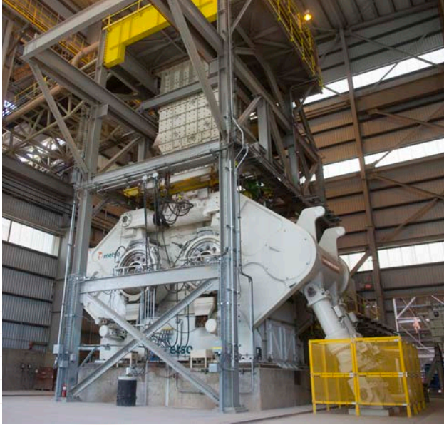
The HRC 3000 at Morenci is the largest high pressure roll crusher in the world. It is estimated to consume 14 percent less power per ton than traditional HPRC's. High pressure roll crusher technology is being deployed as a highly energy efficient means of crushing ore compared to traditional mill circuits.
