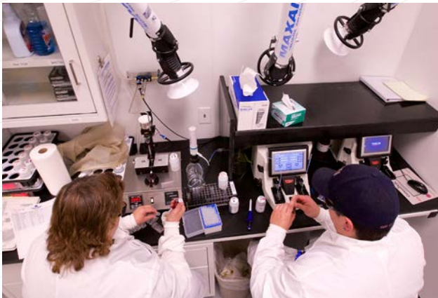
Hundreds of used oil samples are analyzed daily at the company's Oil Analysis Lab and Reliability Center. Technicians prepare samples for an analytical ferrograph instrument that separates wear and contaminant particles from fluid samples that can help mechanics maintain high-efficiency machinery.
